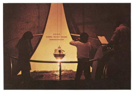
Simulated moon landing craft powered by a hybrid rocket engine.
