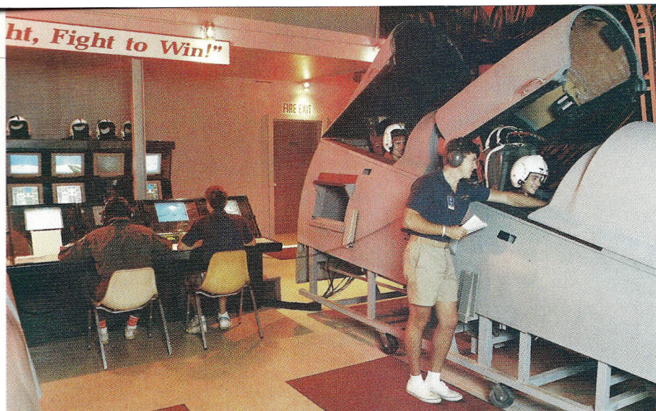
Trainees are instructed in precision aerobatics using one of the high fidelity flight simulators.
